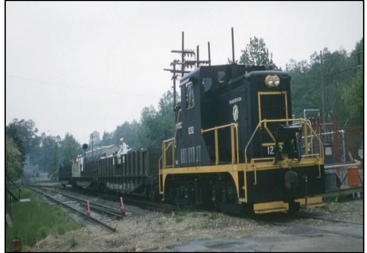
U.S. Army Transportation Corps locomotive #1232 shuttles a train of Navy personnel around inside Picatinny Arsenal in August of 1960. This DE44 locomotive, built in 1953 by the Davenport Locomotive Works in the firm's namesake city in Iowa, was subsequently sold to Cargill (a nationwide agricultural company) during the military's 1960s equipment purge. It survived into the early 2000s at a grain mill in Alta, Iowa, but its disposition beyond that point is unknown. (Note: I believe this image is taken along the north side of Picatinny Lake, looking roughly east. Anyone with better information as to the exact location, I'd love to hear from you!) (The Garbely Publishing Company collection)
