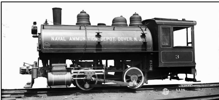
U.S. Navy 0-4-0T steam locomotive #3 was built by the Baldwin Locomotive Works of Eddystone, PA (a suburb of Philadelphia) in 1918 for use at the Naval Ammunition Depot in Dover, NJ, otherwise
