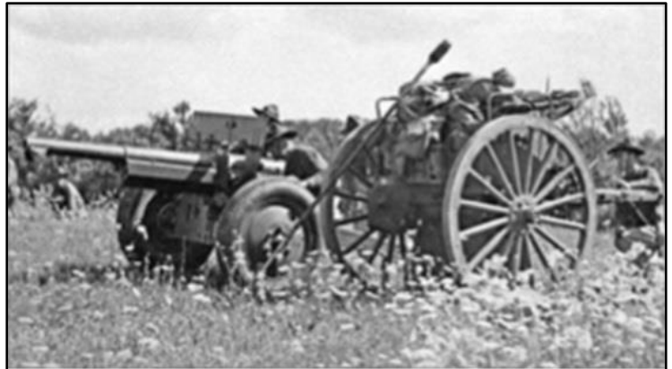
One Gun for Father and Son: A modernized 75mm gun M1897A4 on maneuvers in New York state, 1935. It would not be until the outbreak of war that the Army finally retired the venerable "French '75."
