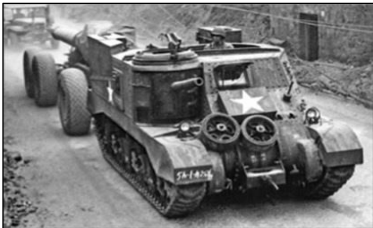
An M33 prime mover, an expedient based off the M31 Tank Recovery Vehicle (itself based off the hull of the M3 medium tank), towing a 240mm howitzer in Italy in January 1944. These vehicles were used as a stopgap until delivery of the M6 HST.
