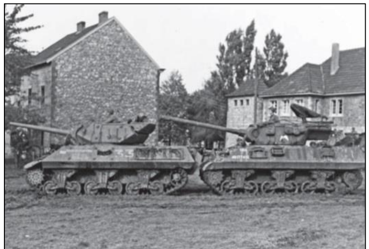
Old and New: The M10 Tank Destroyer, mounting a 3-inch gun, at left; the M36 Tank Destroyer, mounting a 90mm gun, at right. Delivery of the latter was expedited following exposure to the Mark V "Panther" tank
