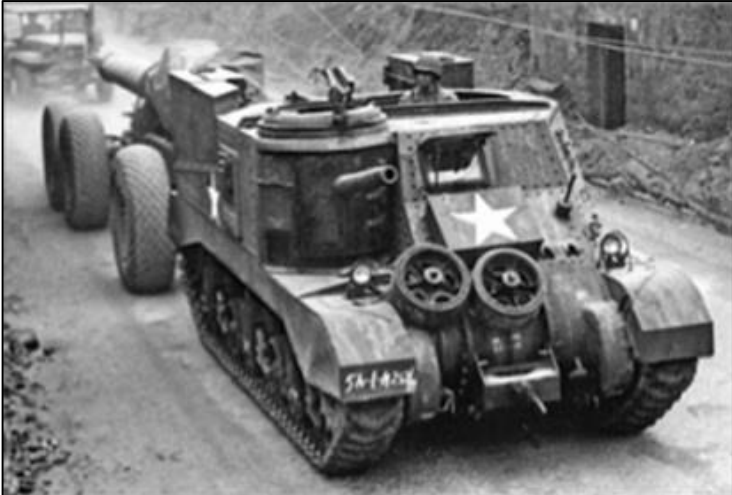
An M33 prime mover pulls a 240mm howitzer in Italy in January 1944. The M33 was a stopgap measure until the M6 HST arrived
