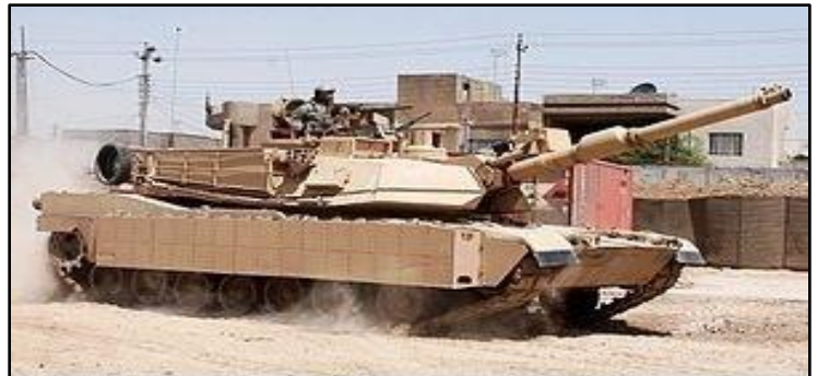
U.S. Army M1A2 Abrams with production TUSK with explosive reactive armor package installed.
