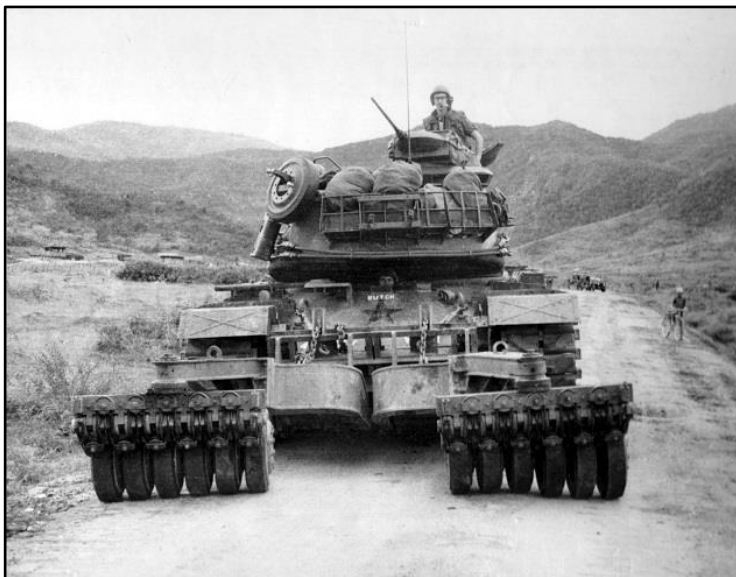
This M48A3 equipped the ENSURE 202 mine roller was operating on Route 19 in August 1970. The name "Butch" is painted in front of the driver's hatch and note the star on the front hull was over painted black.
