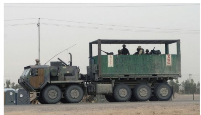
The biggest gun-truck on record in Iraq was created as a conversion of the PLS truck, very similar to the HEMTT, only with two more wheels and a pallet platform. On this platform, the soldiers have installed an armored superstructure with carriages for heavy 12,7 mm M2HB machine-guns and automatic grenade launchers Mk 19.
