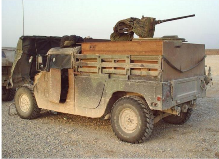
A typical gun-truck on the HMMWV basis, basic version M998. The vehicle is equipped by armor plates, creating a secure space for the soldier up to the driver’s cabin. Armor also creates provisory driver and passenger doors and the car is as well mounted with a heavy 12,7 mm machine-gun Browning M2HB.
