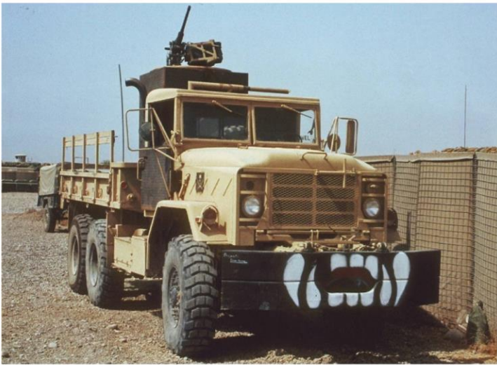
But the US Army infantry is not the only one who uses self-improved gun-trucks. The Special Forces use them as well, as seen on this picture of a M925A1 truck, which belongs to the Fifth Unit of the Special Forces. We can see not only the armored driver's cabin and the 12,7 mm M2HB machine-gun turret, but also an unusual reinforced bumper as well.
