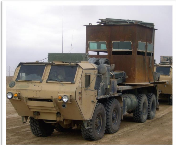
The 8-wheel trucks called HEMTT were also converted into these armored improvisations. This specimen's loading platform was upgraded by a „tower“, enabling firing in all directions. It can be assumed that a vehicle modified in this way was used as a patrol car in dangerous areas.
