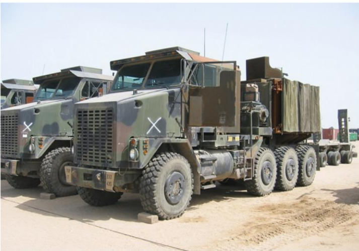
Among the lesser-known vehicles of the US Army, there are the HETS trucks. Every one consists of an 8-wheel truck M1070 and a semi-trailer M1000. And the M1070 trucks became objects of conversion to gun-trucks as well. This specimen got an armored superstructure with two carriages for the 12,7 mm Browning M2HB machine-guns.
