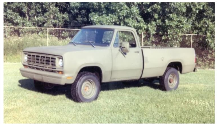
The base vehicle for the M880 series pickup. The position of the parking lights under the headlights identifies this as being built prior to August 15, 1976. After that date the parking lights moved inboard of the headlights.
